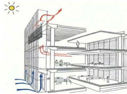
Fig. 1. One type of double skin facade function (<http://cajaislant.com/blog-cajaislant/>, 2018)
