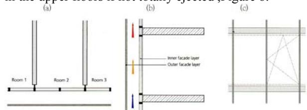
Fig. 8. Multistory DSF: Plan (a); section (b) and elevation(c) (Osterle, 2001)
