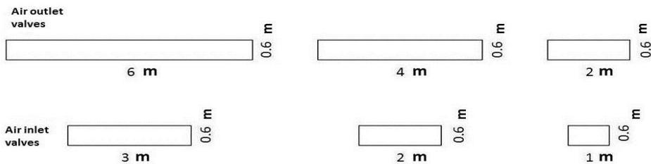
Fig.15. Three different types of air inlet and outlet valves at a ratio of 1 : 2 (Authors,2017)
