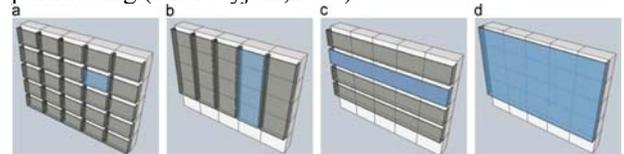
Fig. 3. DSF classification: (a) Box Window, (b) Shaft-Box(c)Corridorand(d)Multi-Storey Double'Skin Facade. (Azarbayjani,2010)
