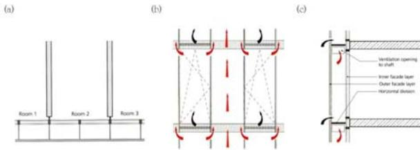
Fig. 5. Shaft box facade: Plan (a), section (b) and elevation(c) (Osterle, 2001)
