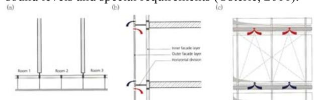
Fig. 4. Box-window type: Plan (a); section (b); elevation(c) (Osterle, 2001)
