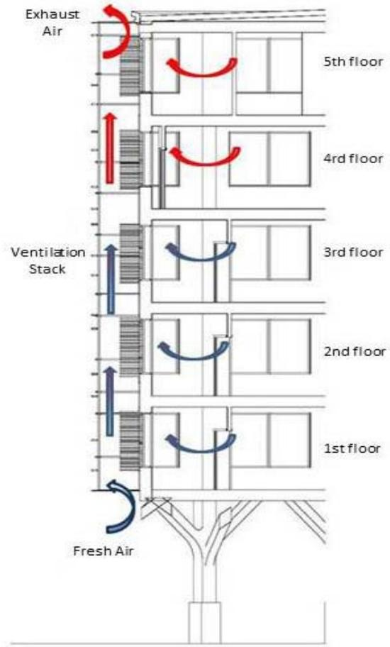
Fig.11. Section of Double skin facade for simulation (Authors, 2017)
