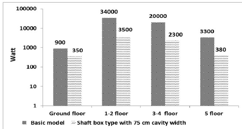
Fig. 25. Comparing direct solar gain both cases of basic – model without DSF and the superior case (Authors, 2017)
