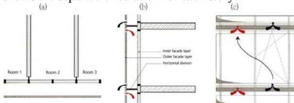
Fig. 7. Corridor facade: plan (a); section (b) and elevation (c) (Osterle, 2001)
