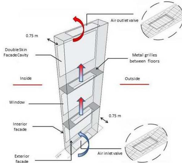
Fig.14. one of the different types of air inlet and outlet valves at a ratio of 1 : 1 in double skin facade – shaft box type. (Authors,2017)
