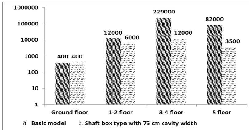
Fig. 24. Comparing indirect solar gain in both cases of basic model without DSF and superior case (Authors,2017)
