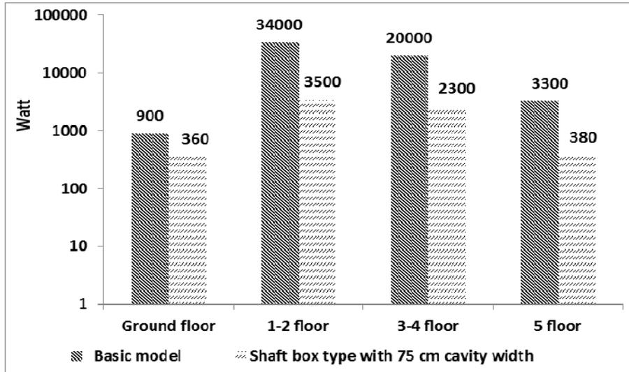
Fig.21. Comparing direct solar gain in both cases of basic – model without DSF and superior case (Authors, 2017)
