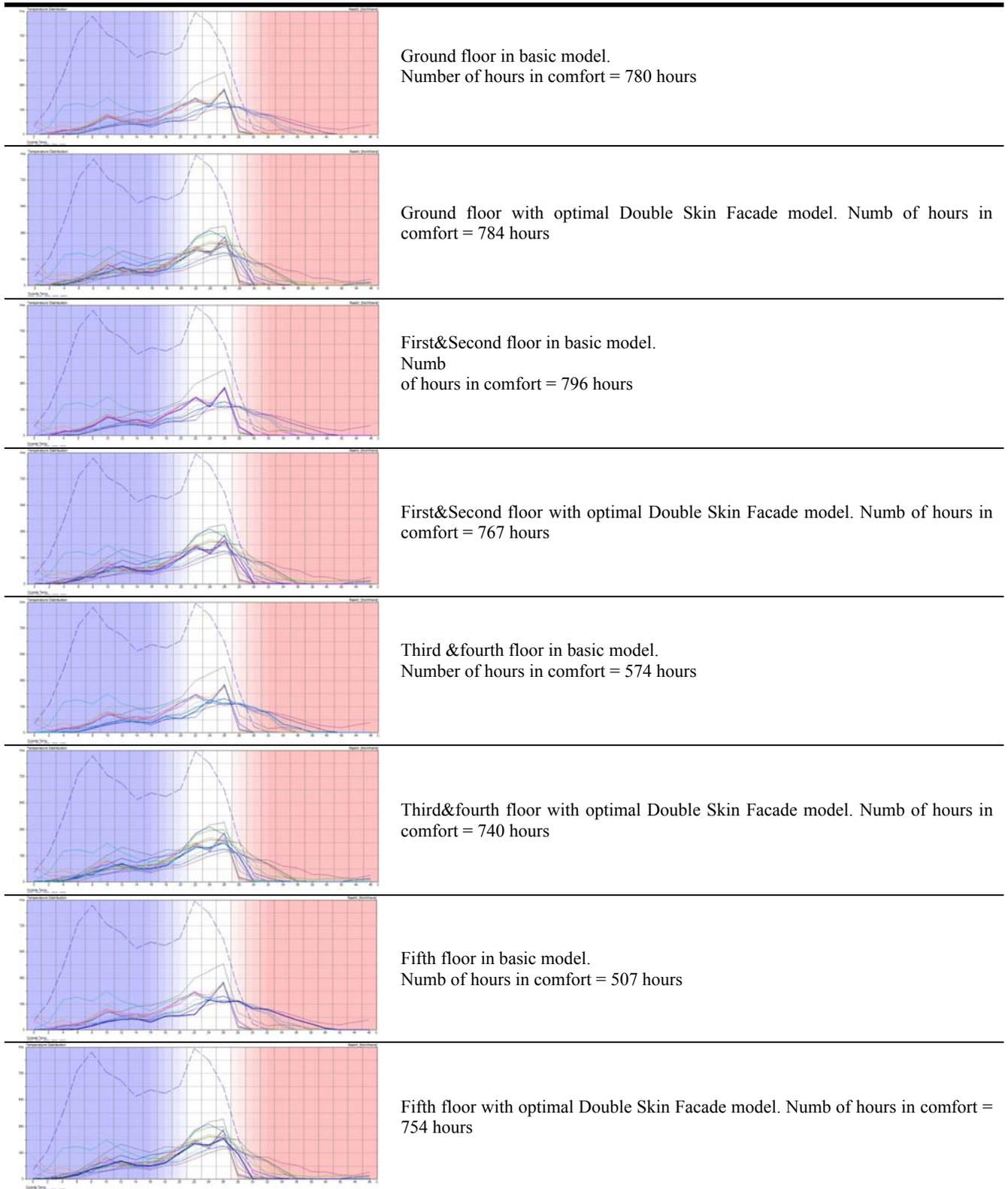
Fig. 22. Comparison of temperature distribution diagrams of different building floors in basic model with optimal Double Skin Facade model for the second six months of the year (autumn and winter) (drawing, Ecotect).
