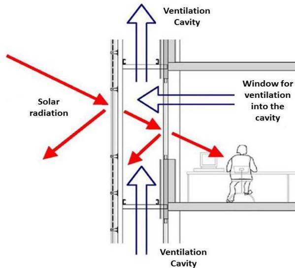
Fig. 17. Section of optimum Double skin facade proportionate to Rasht climate (Authors,2017)
