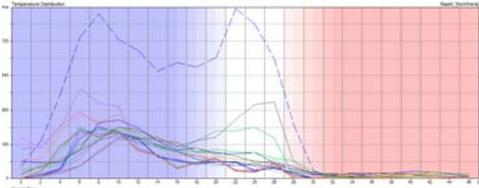
Ground floor with optimal Double Skin Facade model. Number of hours in comfort = 152 hours
