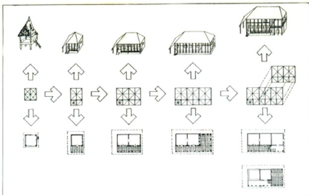
Fig. 9. Expansion pattern of the base unit in construction in Gilan (Diba and Yaghini, 1993)
