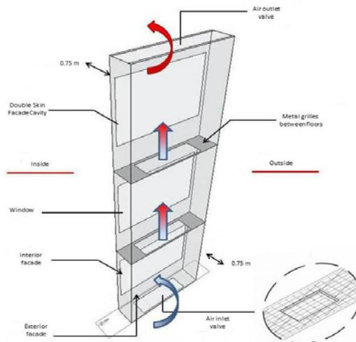
Fig.16. One of the different types of air inlet and outlet valves with ratio of 1 : 2 in double skin facade – shaft box type (Authors,2017)
