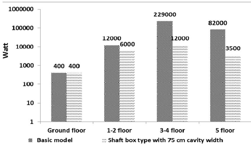
Fig.20. Comparing indirect solar gain in both cases of basic-model without DSF and superior case (Authors, 2017)
